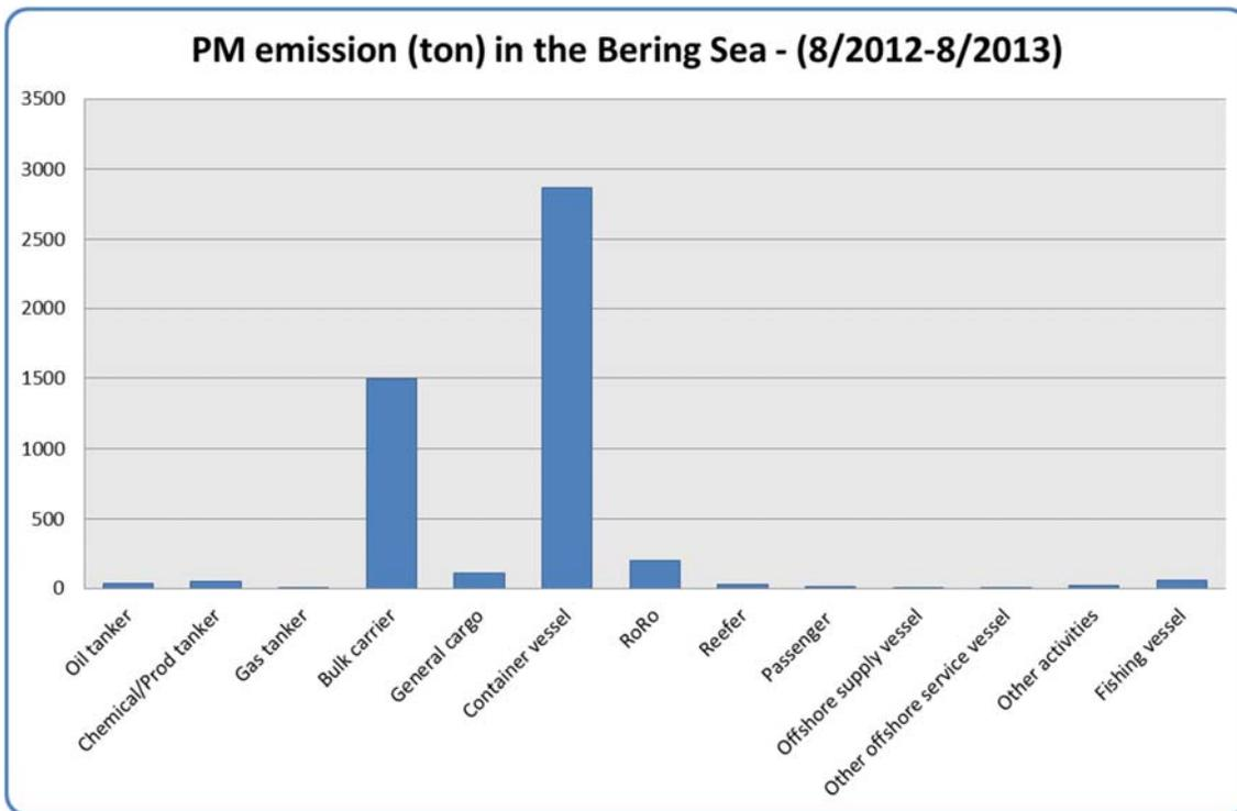
Figure 5-5 - PM emission between vessel categories
