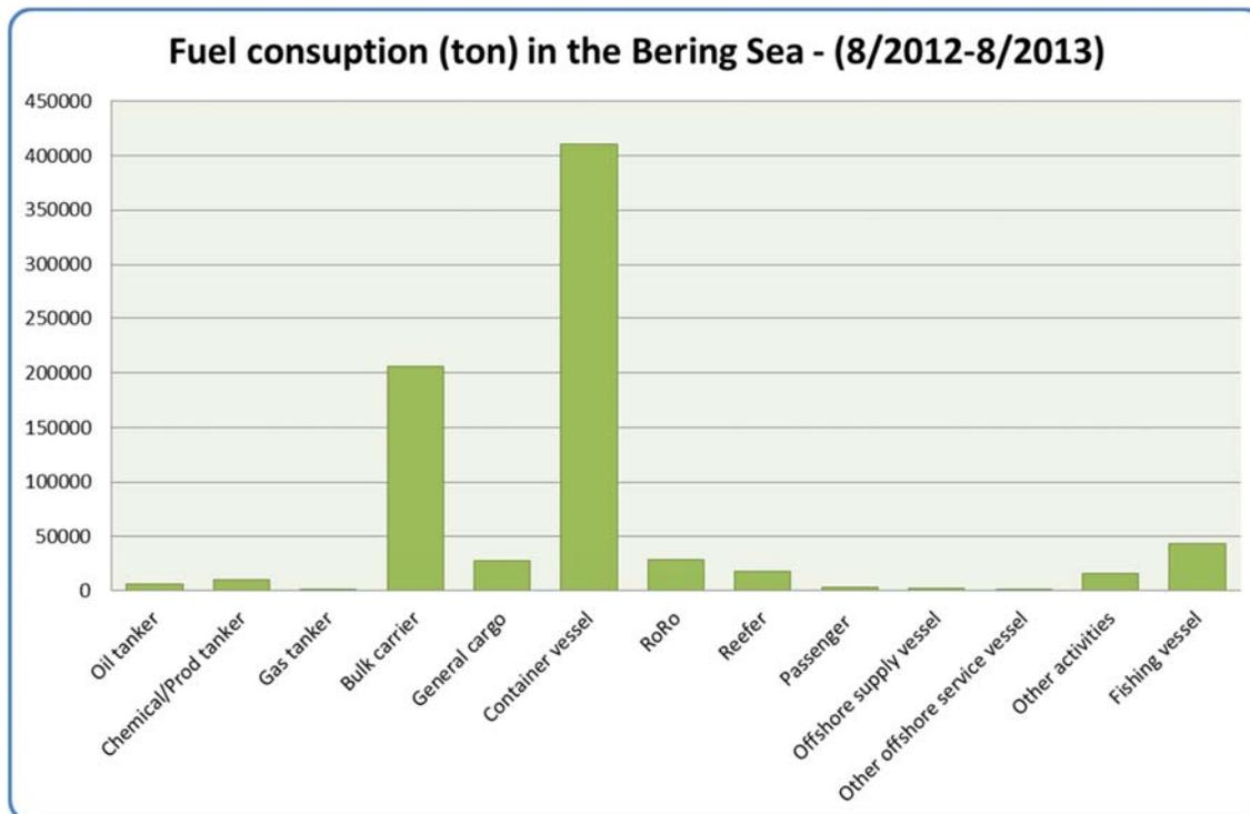
Figure 5-1 - Fuel consumption between vessel categories
