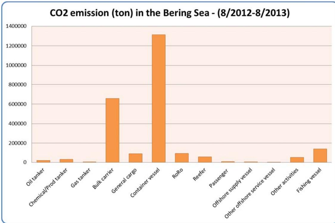
Figure 5-2 - CO2 emission between vessel categories
